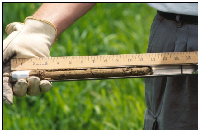
Figure 1: PSNT samples need to be taken over 12 inch depth when the corn is 6-12 inches tall to provide an accurate prediction of nitrate availability from organic N.
