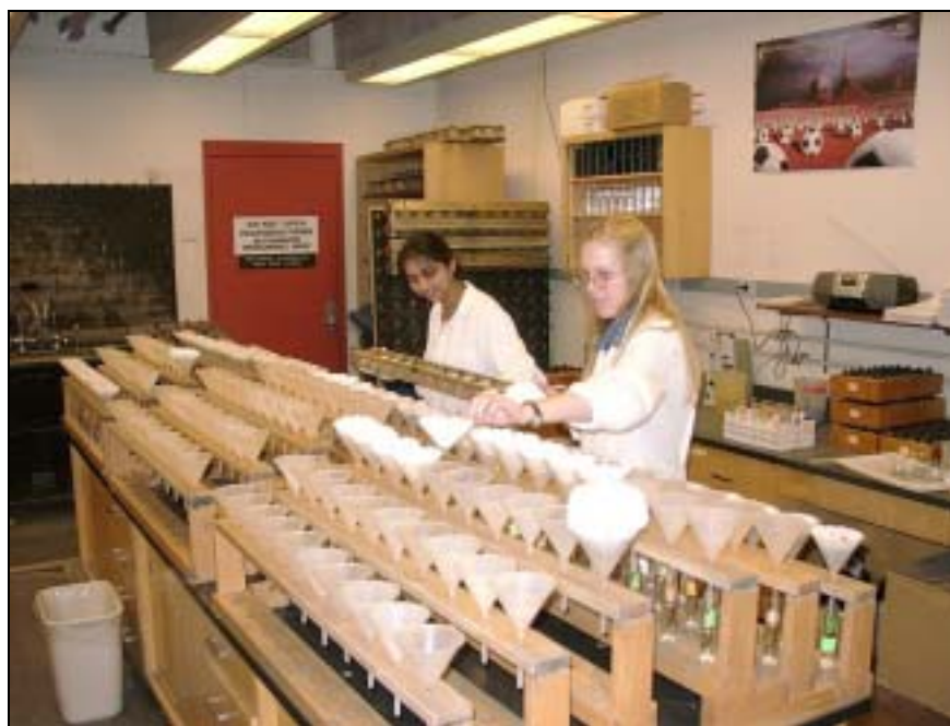
Figure 2: Soil samples are analyzed for pH, organic matter, nitrate and Morgan extractable P, K, Ca, Mg, Fe, Al, Mn, and Zn in the Cornell University Nutrient Analysis Laboratory. Brookside Laboratories Inc. and Spectrum Analytic Inc. analyze the samples for pH, Mehlich-III extractable nutrients and Bray-1 P.
