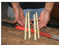
Quartering is a quick and easy way to ensure that a quality sample arrives at the laboratory.
