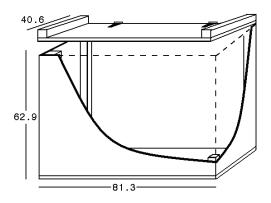
dimensions of the boxes are 81.3 cm in length, 40.6 cm in width, and 62.9 cm in height (see diagram). A 19 by 25 mm hole was cut into the side of the box for electrical plug of the griddle. Inside corners and sides of the top of the lid were secured with 38 by 38 mm spruce lumber. The bottom of the lid was lined with 32 by 5 mm weather stripping (Prod. No. V447, Thermwell Products Co., Mahwah, NJ).
