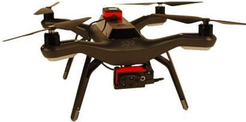
Figure 8: Drone-mounted NDVI and multispectral cameras can be used to quickly obtain scans of fields.
