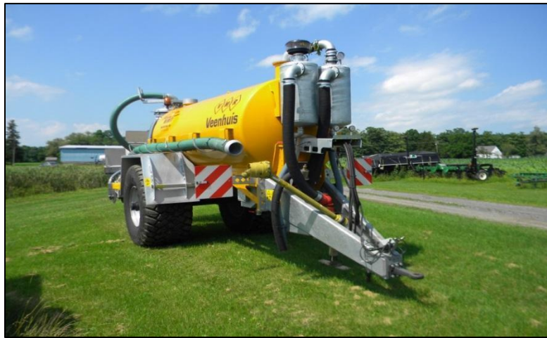
Figure 12. Tanker-mounted Veenhuis liquid manure injector which was used in trials in Aurora.
