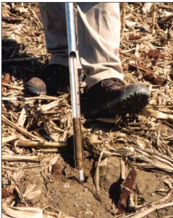
Generally, you'll get more accurate phosphorus estimates with three soil cores per acre when soil sampling.
