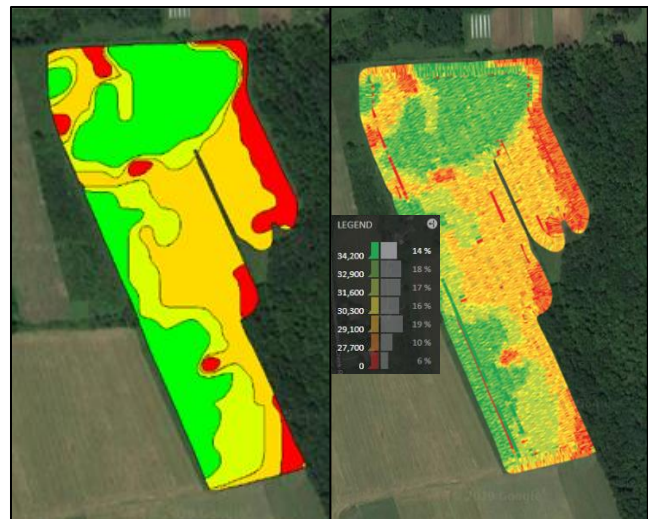
Figure 1. Yield stability zones defined using SMS Ag Leader (left) and variable rate seeding based on the zones (right).
