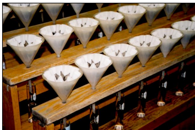
Figure 1: In the laboratory, soils are extracted with a chemical extraction solution, the mixture is filtered and P concentrations in the solution are measured.
