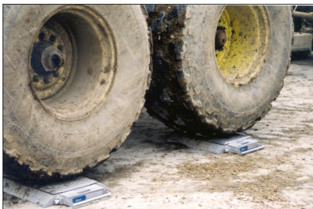
Figure 1: With portable scales, weigh each axle separately.
