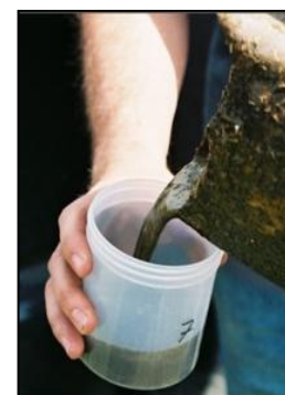
Figure 2: Fill sample container 2/3 rd s full and freeze sample.
