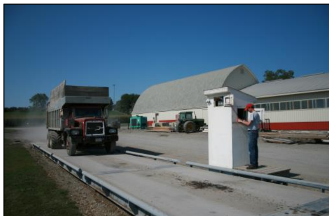
Figure 2: Using farm scales to track yield and crop inventory.
