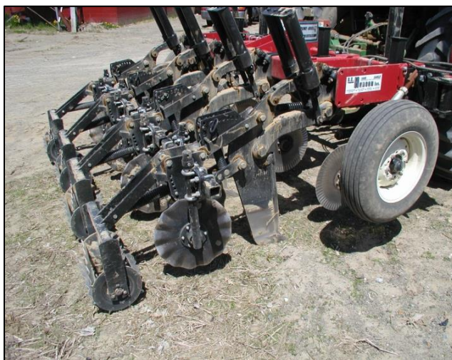
Figure 2: Zone builders typically have the same set of core components: cutting coulters, deep shanks, hilling coulters, and rolling baskets.
