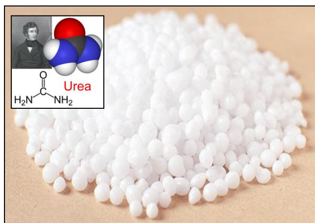
Figure 2: Urea fertilizer is a popular nitrogen fertilizer choice for farmers due to its high nitrogen content per unit material (46%), low cost per unit nitrogen, ease of storage and suitability for use in solid or liquid formulations.
