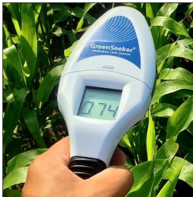
Figure 1: Handheld sensor displaying the NDVI value reflected by the plant canopy.
