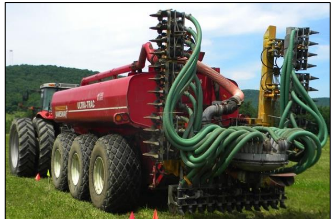
Figure 1. Tanker-mounted shallow disk injector unit without additional coulters to cover the slits.
