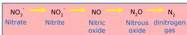
Figure 1. Denitrification, a natural process, is the primary cause of nitrous oxide emissions from crop fields.
