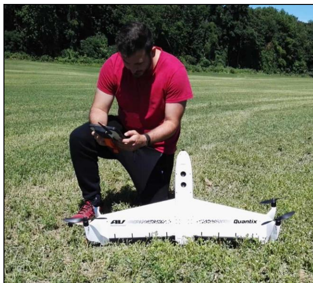
Angel Maresma sets up Quantix for its fully automated flight over a neighboring corn field, measuring true color and near-infrared multispectral light reflected from the leaf canopy and soil.
