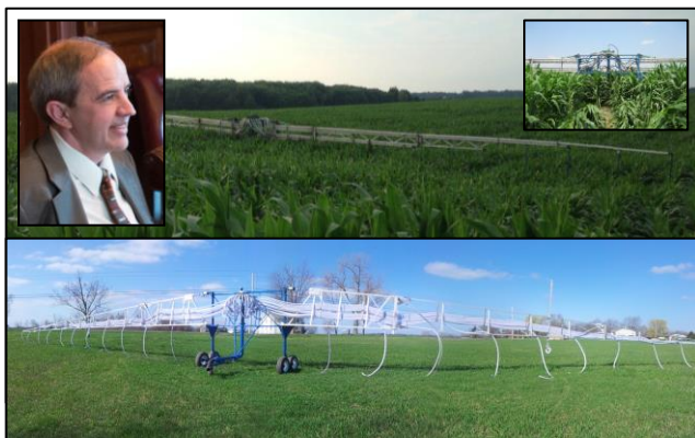
Spruce Haven Farm and Cuff Farm Services’ “Nutrient Boom” delivers manure to the surface of the ground in growing crops through flexible hoses attached to a boom applicator.
